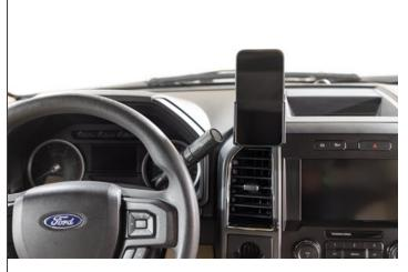
7. The ProClip Mount is in place. Example device holder shown without extension plate.
