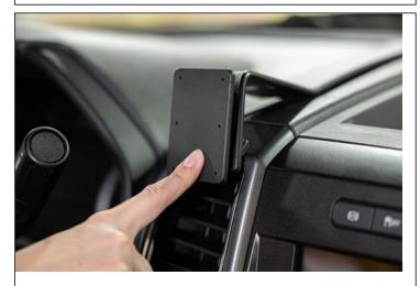
3. **Installing the Mount:** Apply pressure on the lower part of the ProClip face plate to make sure the tape adheres to the dash trim.
