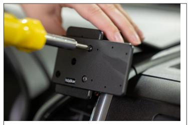
5. **Installing the Optional Extension:** Use the included self-tapping screws to attach the extension plate to the mount face.
