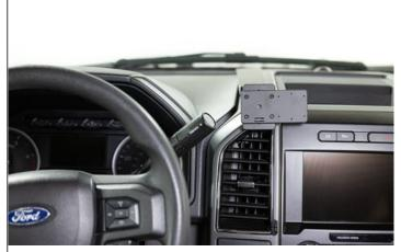
6. The ProClip Mount is in place with extension plate.
